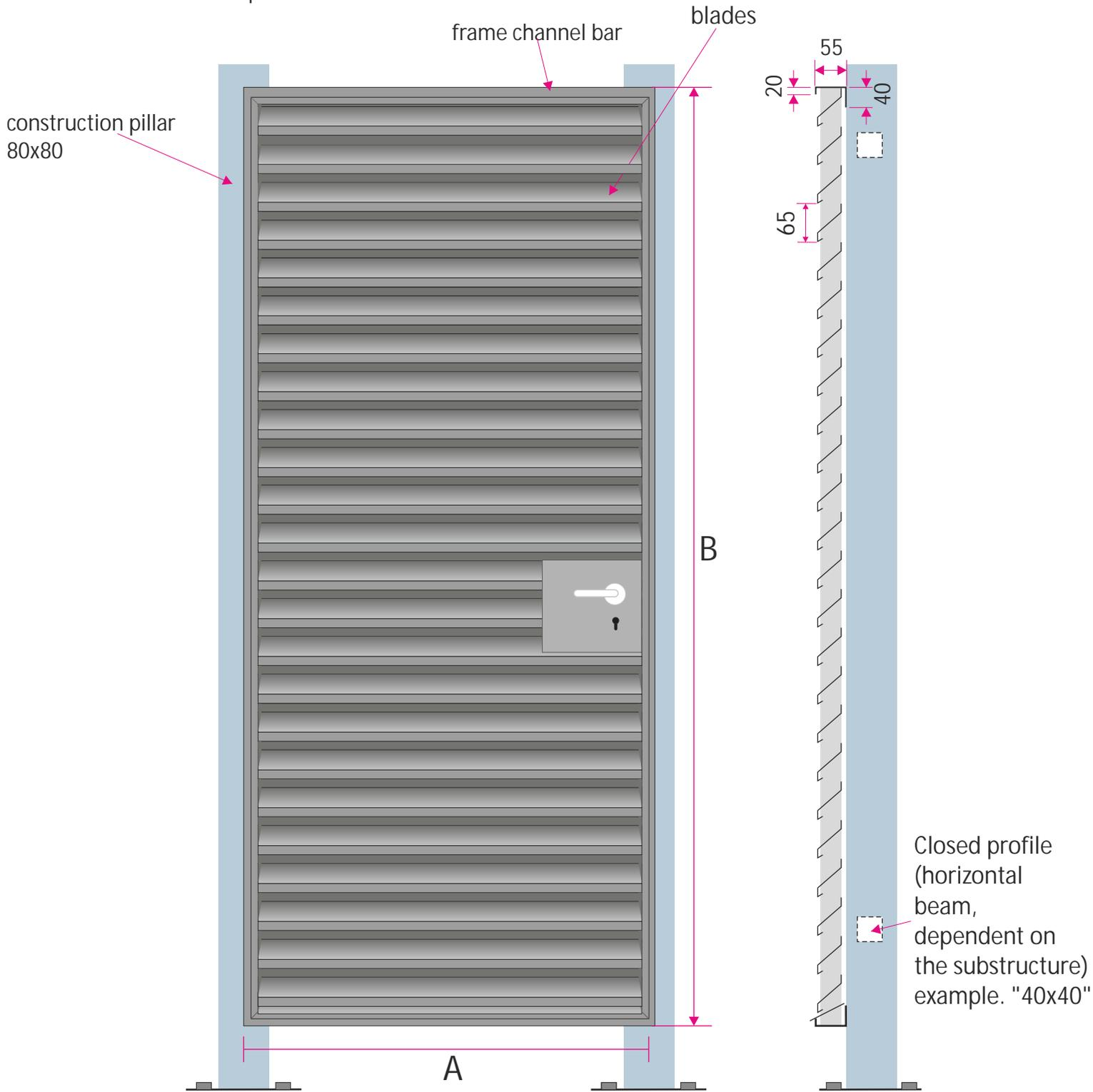
vertical closed profile (depending on the substructure)
