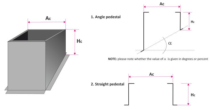
The height of the straight and angle pedestal adjusted to the conditions at its mounting location (need to define at the time of making order).
