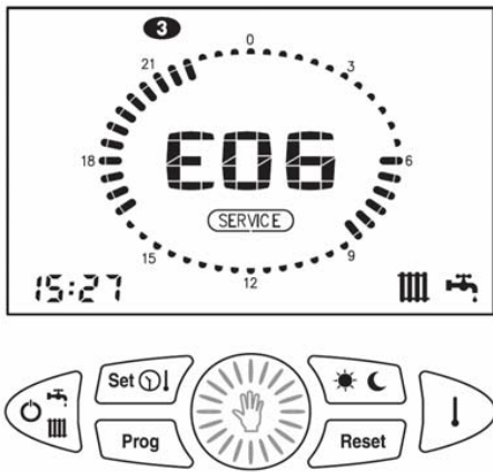
Figure 12.2 Non resettable fault
