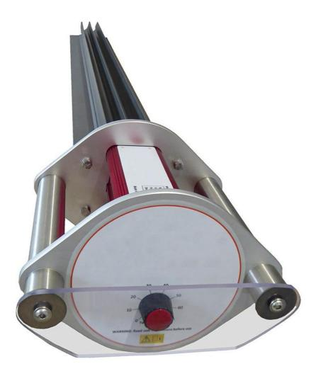
The device is powered by 240Vac and contains a unique heating system which uses a Thermal Transfer System (TTS) to ensure even distribution of heat across the product's heating surface, even when semi-submerged. This prevents the formation of hot spots across the heating surface as the IBC empties, ensuring no burning or discoloration of the fluid.<sup>4</sup>
