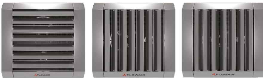
LEO INOX fan heaters can be installed in any position on vertical and horizontal surfaces. They are equipped with air blades, which can be installed vertically or horizontally in air outlet. This solution makes possible to direct stream in any direction.
