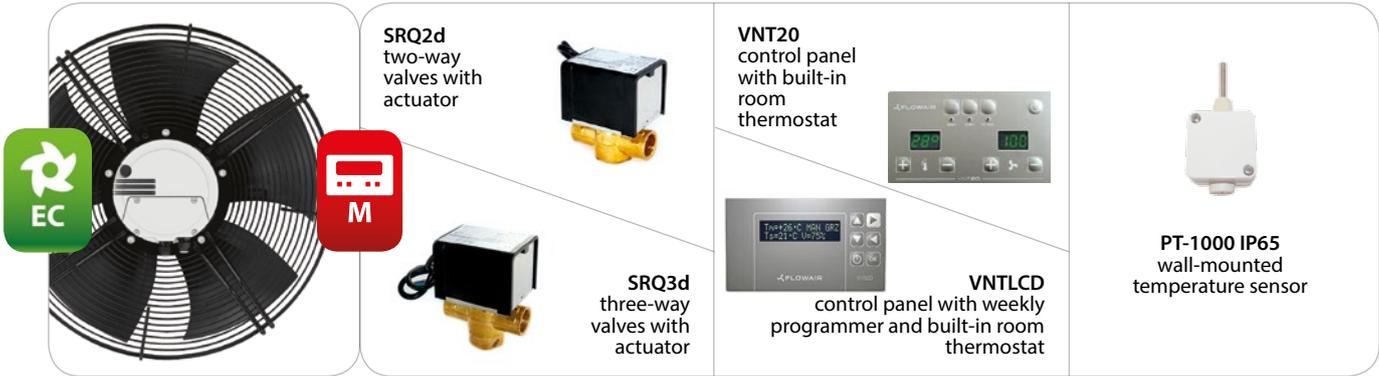
It is an energy-efficient heating system prepared for buildings with medium and big cubic measure. Airflow and heating capacity are automatically controlled depending on actual temperature - air flow is adjusted to current heat demand. Control panel (VNTLCD or VNT20) automatically and steplessly changes the speed of the fan according to the difference between air temperature set on panel and measured by air temperature sensor.
