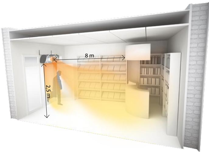
Air curtain range defines the maximum height of installation. For ELIS DUO it is 2,5 m - on this height the fan heater section has an 8 m range.
